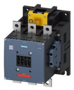
Power contactor, AC-3 300 A, 160 kW / 400 V Coil AC 50/60 Hz and DC 96-127 V x (0.8-1.1) F-PLC input 24 V DC 3-pole size S10 Auxiliary contacts 2 NO + 2 NC cannot be dissolved (SUVA) Main circuit: Busbar Control and auxiliary circuit: screw terminal
