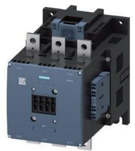
Power contactor, AC-3 500 A, 250 kW / 400 V AC (50-60 Hz) / DC 110-127 V UC Auxiliary contacts 2 NO + 2 NC 3-pole, size S12 Busbar connections Operating mechanism: conventional Spring-type terminals
