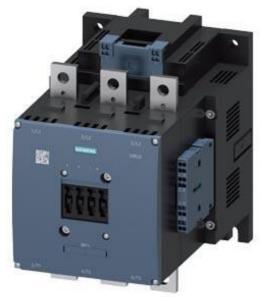
Power contactor, AC-3 500 A, 250 kW / 400 V AC (50-60 Hz) / DC 240-277 V UC Auxiliary contacts 2 NO + 2 NC 3-pole, size S12 Busbar connections Operating mechanism: conventional Spring-type terminals
