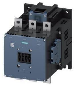
Power contactor, AC-3 500 A, 250 kW / 400 V AC (50-60 Hz) / DC 200-220 V UC Auxiliary contacts 2 NO + 2 NC 3-pole, size S12 Busbar connections Operating mechanism: conventional screw terminals
