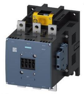
Power contactor, AC-3 500 A, 250 kW / 400 V coil AC 50/60 Hz and DC 96-127 V x (0.8-1.1) F-PLC input 24 V DC 3-pole size S12 auxiliary contacts 2 NO + 2 NC main circuit: busbar Control and auxiliary circuit: screw terminals
