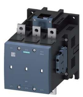
Vacuum contactor, AC-3 400 A, 200 kW / 400 V AC (50-60 Hz) / DC operation 200-277 V UC Auxiliary contacts 2 NO + 2 NC 3-pole, Size S12 Busbar connections Drive: electronic with PLC interface 24 V DC
