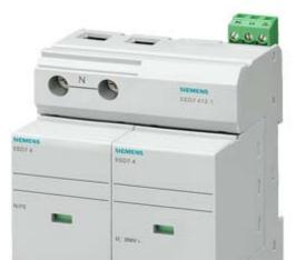
Lightning arresters, type 1 Requirement class B, UC 350V Pluggable protective modules 2-pole, 1+1 circuit for TN-S and TT systems with remote display
