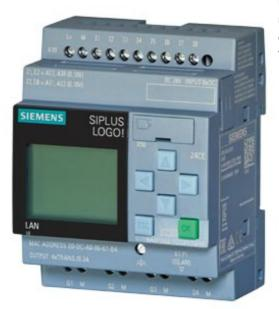
SIPLUS LOGO! 24CE -20...+70°C start up -20°C with conformal coating based on 6ED1052-1CC08-0BA0 . logic module, Display PS/I/O: 24 V/24 V /24 V trans., 8 DI (4AI)/4DO, memory 400 blocks, modular expandable, Ethernet integr. web server, data log, user-defined Web pages, standard microSD card for LOGO! Soft Comfort V8 or higher, older projects executable
