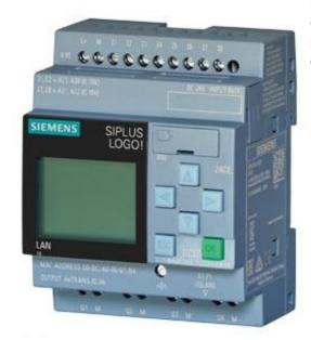
SIPLUS LOGO! 230RCE -20 ... +70°C start up -20°C with conformal coating based on 6ED1052-1FB08-0BA0 . logic module, display PS/I/O: 115V/230V/relay, 8 DI/4 DO, memory 400 blocks, modular expandable, Ethernet, integr. web server, data log, user-defined Web pages, standard microSD card for LOGO! Soft Comfort V8 or higher, older projects executable
