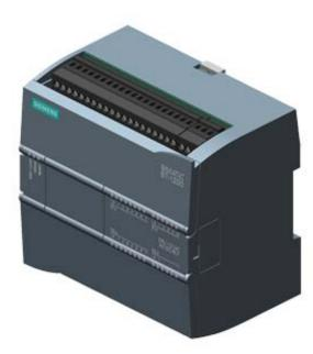
SIPLUS S7-1200 CPU 1214C AC/DC/relay -40...+70 °C with conformal coating based on 6ES7214-1BG40-0XB0 . compact CPU, AC/DC/relay, onboard I/O: 14 DI 24 V DC 10 DO relay 2 A 2 AI 0-10 V DC, Power supply: AC 85-264 V AC @ 47-63 Hz, Program/data memory 100 KB
