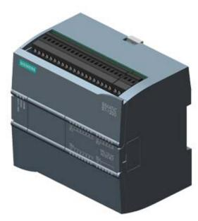
SIPLUS S7-1200 CPU 1214C AC/DC/relay -25...+55 °C with conformal coating Signal board usable based on 6ES7214-1BG40-0XB0 . compact CPU, AC/DC/relay, onboard I/O: "14 DI 24 V DC; 10 DO relay 2 A; 2 AI 0-10 V DC, Power supply: AC 85-264 V AC @ 47-63 Hz, Program/data memory 75 KB
