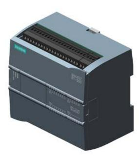
SIPLUS S7-1200 CPU 1214C DC/DC/relay -40...+70 °C with conformal coating based on 6ES7214-1HG40-0XB0 . compact CPU, DC/DC/relay, onboard I/O: 14 DI 24 V DC 10 DO relay 2 A 2 AI 0-10 V DC, Power supply: DC 20.4-28.8V DC, Program/data memory 100 KB
