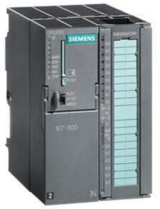
SIPLUS S7-300 CPU 312C with conformal coating according to EN 50155 T1 Cat 1 Cl A/ B based on 6ES7312-5BF04-0AB0 . Compact CPU with MPI, 10 DI/6 DQ, 2 high-speed counters (10 kHz) Integr. power supply 24 V DC, work memory 64 KB, Front connector (1x 40-pole) and Micro Memory Card required
