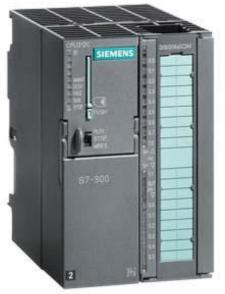
SIPLUS S7-300 CPU 312C for medial exposure -25...+70  $^{\circ}$ C based on 6ES7312-5BF04-0AB0 . Compact CPU with MPI, 10 DI/6 DQ, 2 high-speed counters (10 kHz) Integr. power supply 24 V DC, work memory 64 KB, Front connector (1x 40-pole) and Micro Memory Card required
