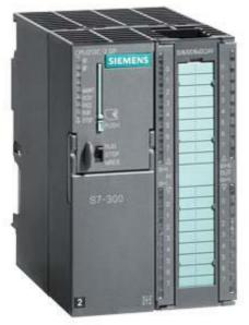
SIPLUS S7-300 CPU 313C-2DP for medial exposure -25...+70  $^{\circ}$ C based on 6ES7313-6CG04-0AB0 . Compact CPU with MPI, 16 DI/16 DO, 3 high-speed counters (30 kHz), integrated DP interface, Integr. power supply 24 V DC, work memory 128 KB, Front connector (1x 40-pole) and Micro Memory Card required
