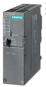
SIPLUS S7-300 CPU 315-2DP -25 ... +60 DEGREES C WITH CONFORMAL COATING ACCORDING EN50155 T1 KAT 1 KL A BASED ON 6ES7315-2AH14-0AB0 . CPU WITH MPI INTERFACE INTEGRATED 24 V DC POWER SUPPLY 256 KBYTE WORKING MEMORY 2. INTERFACE DP-MASTER/SLAVE MICRO MEMORY CARD NECESSARY
