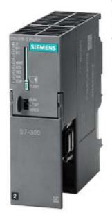
SIPLUS S7-300 CPU315-2PN/DP -25 ... +70 DEGREES C WITH CONFORMAL COATING BASED ON 6ES7315-2EH14-0AB0 . CENTRAL PROCESSING UNIT WITH 384 KBYTE WORKING MEMORY, 1. INTERFACE MPI/DP 12MBIT/S, 2. INTERFACE ETHERNET PROFINET, WITH 2 PORT SWITCH, MICRO MEMORY CARD NECESSARY
