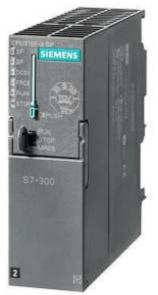
SIPLUS S7-300 CPU 315F-2DP with conformal coating according to EN 50155 T1 Cat 1 Cl A/ B based on 6ES7315-6FF04-0ab0 . Fail-safe module with MPI Integr. power supply 24 V DC, Work memory 384 KB, 40 mm width, 2nd interface DP master/ slave Micro Memory Card required
