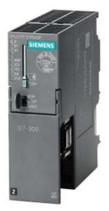
SIPLUS S7-300 CPU 317F-2PN/DP -25...+60  $^{\circ}$ C with conformal coating Based on 6ES7317-2FK14-0AB0 . Central processing unit with 1.5 MB work memory, 1st interface MPI/DP 12Mbit/ s, 2nd interface Ethernet PROFINET, with 2-port switch, Micro Memory Card required
