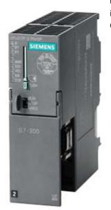
SIPLUS S7-300 CPU 317F-2PN/DP conformity with EN 50155 T1 Kat 1 KI A/B Based on 6ES7317-2FK14-0AB0 . Central processing unit with 1.5 MB work memory, 1st interface MPI/DP 12Mbit/ s, 2nd interface Ethernet PROFINET, with 2-port switch, Micro Memory Card required
