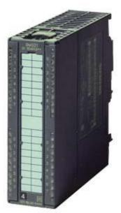
SIPLUS S7-300 SM 321-20-pole -25...+70 °C with conformal coating Conformity with EN 50155 T1 Kat 1 KI A/B based on 6ES7321-7BH01-0AB0 . Digital input Isolated "16 DI; 24 V DC, 1x 20-pole," process interrupt, diagnostics, suitable for isochronous mode operation
