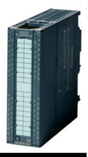
SIPLUS S7-300 SM322 - 20-POLE -25...+70 DGR C WITH CONFORMAL COATING WITH CONFORMITY EN50155 T1 CAT 1 KL A/B BASED ON 6ES7322-1BH01-0AA0 . DIGITAL OUTPUT OPTIC. ISOLATED 16D0, 24V DC, 0.5A, SUM OF CURRENTS 4A/GROUP (8A/MODULE)
