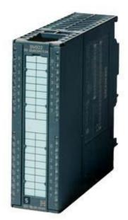
SIPLUS S7-300 SM 322-40-pole -25...+60 °C with conformal coating Conformity with EN 50155 T1 Cat 1 Cl A/B based on 6ES7322-1HF10-0AA0 . Digital output Isolated 8 DO (relay), 1x 40-pole, 24 V DC, 5 A or 230 V AC, 5 A, connectors with spring-loaded terminal can be used as of 6ES7392-1BM01-0AA0
