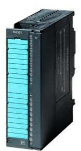
SIPLUS S7-300 SM 331 40-pole -25...+70 °C with conformal coating Conformity with EN 50155 T1 Kat 1 KI A/B based on 6ES7331-7NF00-0AB0 . Analog input isolated "8 AI; +/-5/10 V, 1-5 V, +/-20 mA, 0/4 to 20 mA, 16 bit (55ms), Single rooting (50 V COM.)
