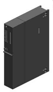
SIPLUS S7-400 CPU 414-3 PN/DP -25 ... +70°C with conformal coating based on 6ES7414-3EM07-0AB0 . Central processing unit with: Work memory 4 MB, (2 MB code, 2 MB data), Interfaces 1st interface MPI/DP 12 Mbit/s, (X1), 2nd interface ETHERNET/PROFINET (X5) 3rd interface IF 964-DP plug-in (IF1)
