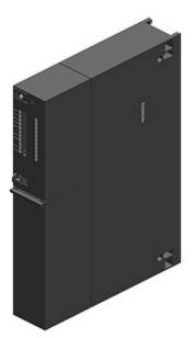
SIPLUS S7-400 CPU 416-3 PN/DP -25 ... +70°C with conformal coating based on 6ES7416-3ES07-0AB0 . Central processing unit with: Work memory 16 MB, (8 MB code, 8 MB data), Interfaces 1st interface MPI/DP 12 Mbit/s, (X1), 2nd interface ETHERNET/PROFINET (X5) 3rd interface IF 964-DP plug-in (IF1)
