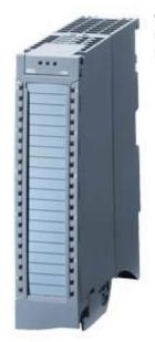
SIPLUS S7-1500 AI 8xU/I HS -40 °C ..+70 °C Start-up -25 °C with conformal coating based on 6ES7531-7NF10-0AB0 . Analog input module AI 8xU/I HS, 16 bit resolution, accuracy 0.4% 8 channels in groups of 8, "Common mode voltage 10 V;" "diagnostics; hardware interrupts" 8 channels in 0.125 ms incl. infeed element, Shield bracket and shield terminal
