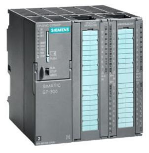
SIMATIC S7-300, CPU 314C-2PN/DP Compact CPU with 192 KB work memory, 24 DI/16 DO, 4 AI, 2 AO, 1 Pt100, 4 high-speed counters (60 kHz), 1st interface MPI/DP 12 Mbit/s, 2nd interface Ethernet PROFINET, with 2-port switch, Integr. power supply 24 V DC, Front connector (2x 40-pole) and Micro Memory Card required
