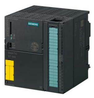
SIMATIC S7-300, CPU 317TF-3 PN/DP, Central processing unit for PLC, Technology and safety tasks, 1.5 MB work memory, 1st interface MPI/DP 12 Mbit/s, 2nd interface DP (drive), 3rd interface Ethernet PROFINET with 2-port switch, Integr. I/O for technology, Front connector (1x 40-pole) and Micro Memory Card min. 8 MB required
