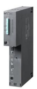
SIMATIC S7-400, CPU 414-3 Central processing unit with: Work memory 4 MB, (2 MB code, 2 MB data), 1st interface MPI/DP 12 Mbit/s, 2nd interface PROFIBUS DP, 3rd interface plug-in IFM module
