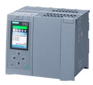
SIMATIC S7-1500, CPU 1518-4 PN/DP MFP, INCLUSIVE C/C++ RUNTIME AND OPC UA RUNTIME LICENSE WORKING MEMORY 4 MB FOR PROGRAM AND 20 MB FOR DATA, 1. INTERFACE: PROFINET IRT WITH 2 PORT SWITCH, 2. INTERFACE: PROFINET RT, 3. INTERFACE: ETHERNET, 4. INTERFACE: PROFIBUS, 1 NS BIT-PERFORMANCE, SIMATIC MEMORY CARD (min. 2 GB) NECESSARY
