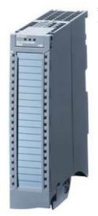
SIMATIC S7-1500, Analog output module AQ 8xU/I HS, 16 bit resolution, accuracy 0.3%, 8 channels in groups of 8, diagnostics, substitute value 8 channels in 0.125 ms oversampling incl. power supply element, shield bracket and shield terminal: Front connector (screw terminals or push-in) separately
