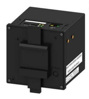
SENTRON, measuring device, 7KM PAC5100, strd mount. rail encl. w/o display, L-L: 690 V, L-N: 400 V, 10 A, strd rail instr., 3-phase, Modbus TCP, apparent /active/reactive energy / cos phi, harmonics: 2. - 40., THD, class 0.5 acc. to IEC61557-12 or cl. 0.5S acc. to IEC62053-22, wide-range pwr sup. unit AC/DC, screw terminals
